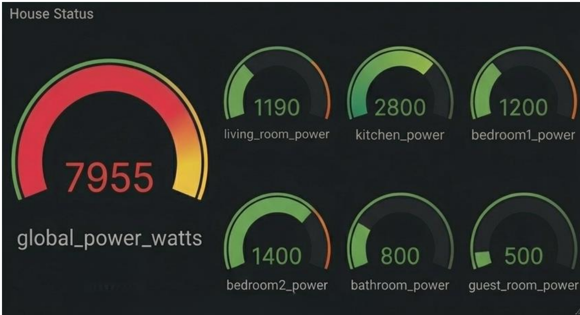
Figure 6. Real-time monitoring dashboard displaying global and per-zone power consumption metrics.
